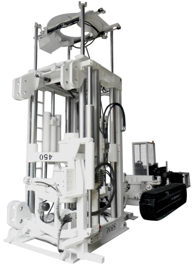
This machine differs from the other ones, because it can drill Boxholes of 28 inches (0.7 m) in diameter and up to a maximum of 196 ft (60 m) in length. It is put on a crawler which moves it and where it can be rotated 180° manually. After that, 2 cylinders set the machine up. Finally, a chute is installed to protect the machine and deflect the chips.
